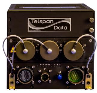
The Removable Memory Module, RMM, consists of 1 to 3 drives in a single carrier supporting recording bandwidths to 1.5GBps and up to 48TB. With data security and throughput in mind, 3 independent data paths (from inputs to disks) allow individual data channels to be written to individual drives. Each carrier includes a built-in power and a 10GE download port eliminating the need for expensive, standalone debrief stations.
